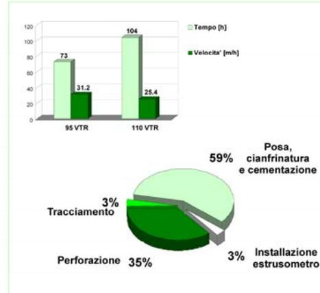
Figure 6 Ground reinforcement times
