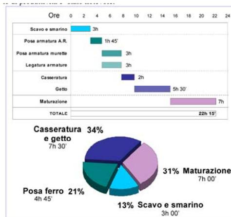
Figure 12 Tunnel invert construction times
