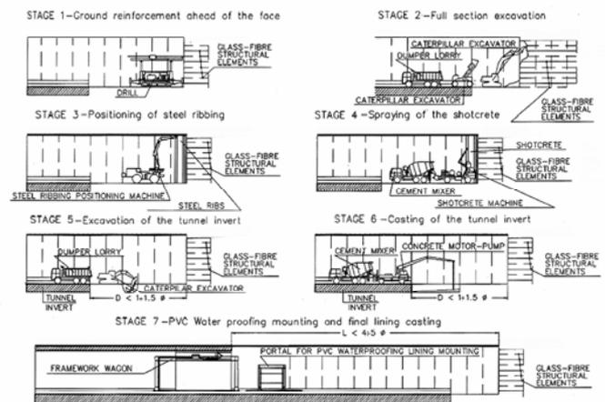
Figure 1. Typical tunnel construction stages
