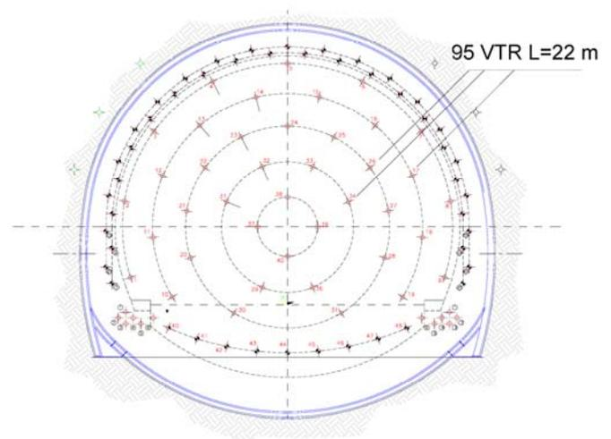
Figure 2 Geometrical layout of the fibre glass elements
