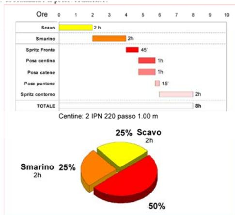
Figure 10 Excavation and preliminary lining times
