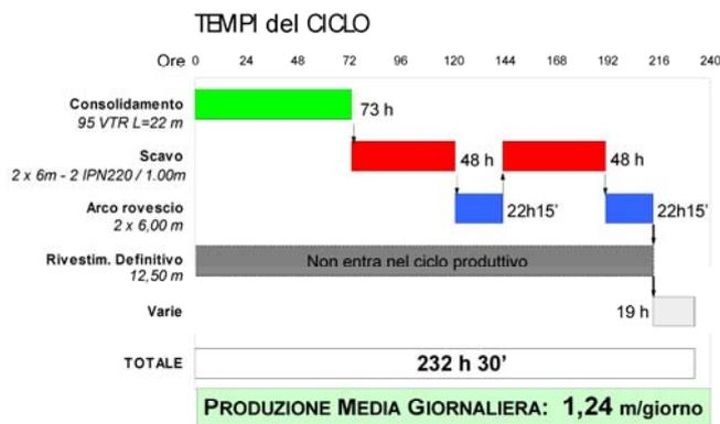
Figure 13 Work cycle times in the initial period
