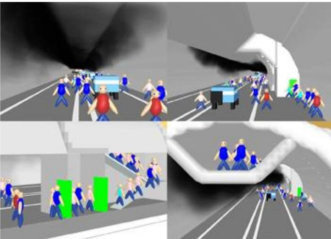
Figure 12. Simulation of escape scenarios in case of fire in the tunnel with Suspended Escape Route
