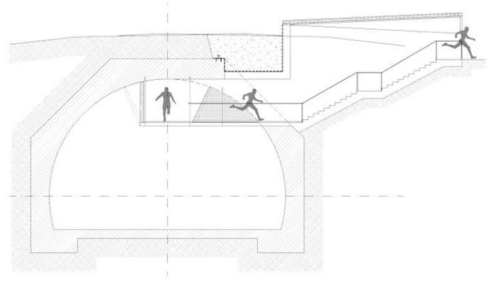
Figure 9. Exit corresponding to the entrances of Sellero tunnel
