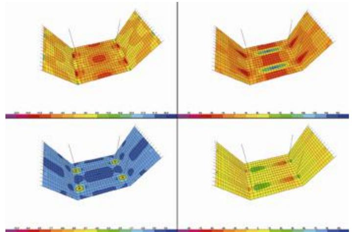
Figure 6. FEM analysis of precast segments
