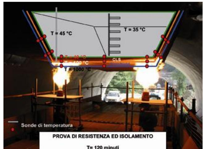
Figura 14. Results of the fire resistance test
