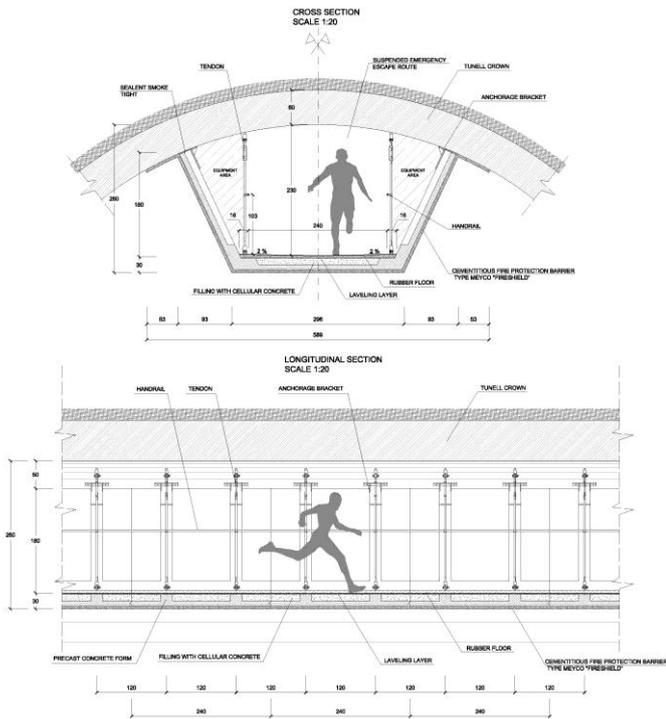
Figure 5. Profile and section of the suspended walkway
