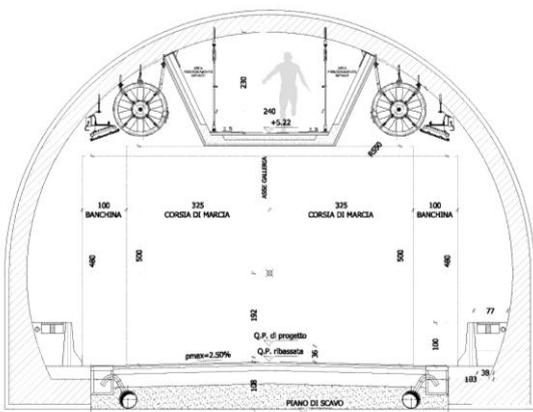
Figure 17. Cross section of Serralunga tunnel line adequate with the Suspended Emergency Escape Route
