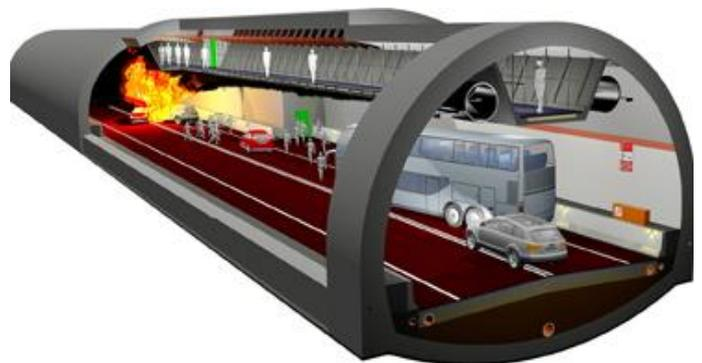
Figure 1. The Suspended escape route in a fire scenario in the tunnel
